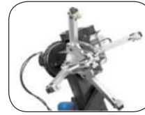
Clockwise and anticlockwise rotation of the clamp range from 14"-26", 14"-56" for 10189941
