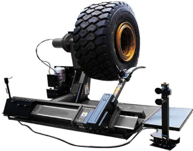
Clockwise and anticlockwise rotation of the clamp range from 14"-26", 14"-56" for 10189941
